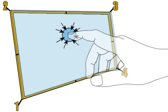
Figure 6.5-2: Four Press Sensing Connections, Quadrant-segmented CDS
