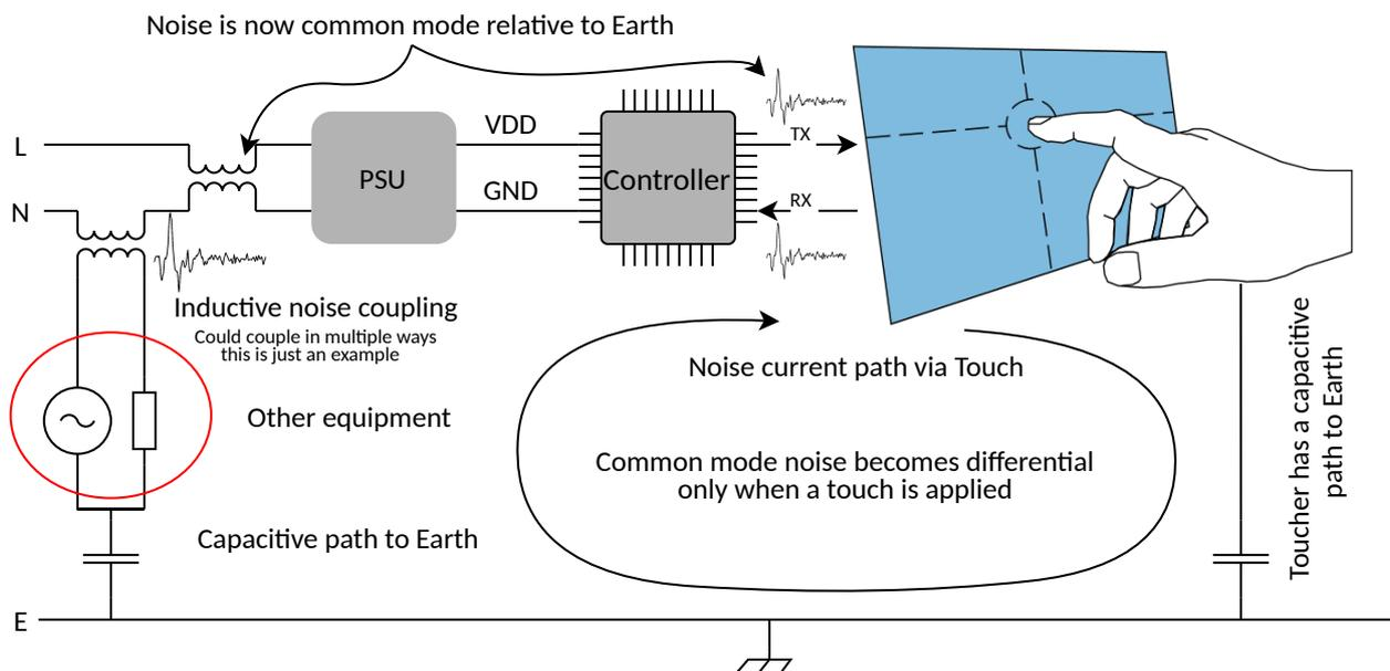
Figure 6.7-1: Example Common Mode Noise From “Other” Equipment
