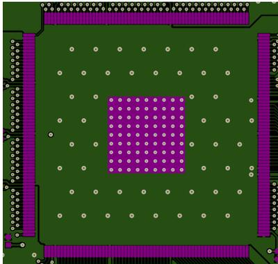
2. The center pad must have a minimum of 25 off, 0.3mm diameter, plugged<sup>40</sup> vias connecting to GND floods on the layers below.
