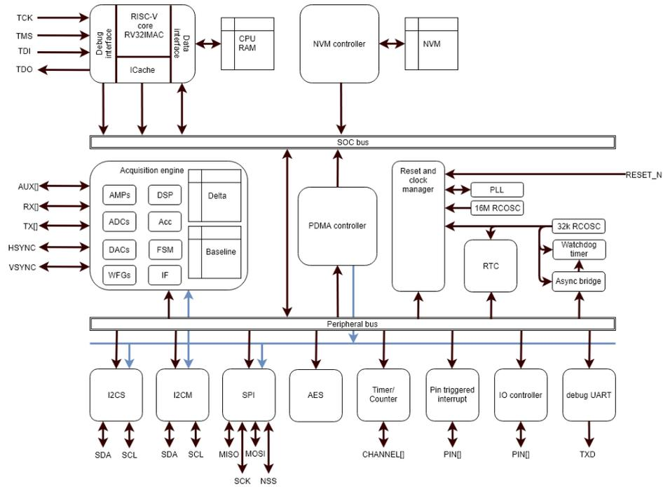
Figure 6.1-2: Simplified System Architecture
