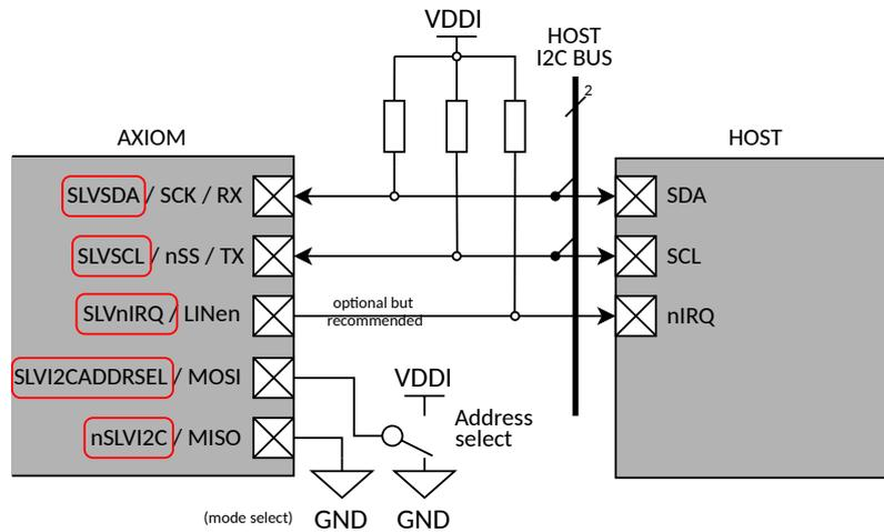
Figure 7.3.2-1: Slave I<sup>2</sup>C Connections
