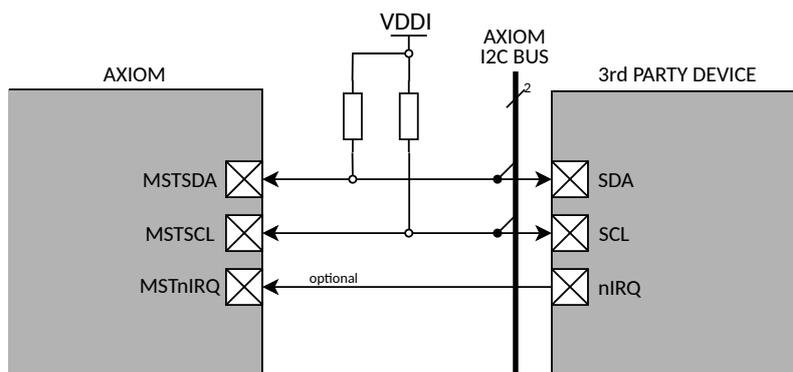
Figure 8-1: Master I<sup>2</sup>C Connections to 3<sup>rd</sup> Party Device(s)
