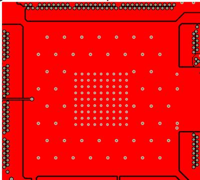
7. Extend a copper GND flood from underneath the body, past the non-sensing pins (i.e. predominantly on one package edge) on the bottom layer of the PCB, to create an extra area of at least 25mm x 25mm. Keep this area wide and continuous and avoid adding narrow necks or meanders, so that the area functions as a good thermal conductor away from the device.
